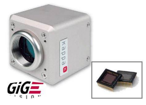
Kappa introduces a new vision camera based on our modular high-performance platform with 14-bit digitization. The first model, the Zelos-655 has a GigE Vision interface and offers a resolution of 2448 x 2050 pixel and a frame rate of up to 9 fps. It fulfills all typical Kappa quality characteristics regarding hardiness and longevity.
