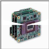
Kappa introduces a new vision camera based on our modular high-performance platform with 14-bit digitization. The first model, the Zelos-02150 has a GigE Vision interface and offers a resolution of 1920 x 1080 and a frame rate of up to 30 fps. It fulfills all typical Kappa quality characteristics regarding hardiness and longevity.
