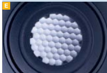
Fly-eye lens for homogeneous fluorescence illumination
