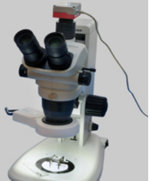
Moticam 2500: with binocular microscope SZ61TR, Nikon Stand C-LEDS and Ryf NKL18 illuminator, including HP Workstation and Eizo 21" screen
