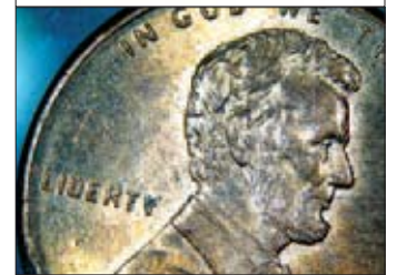
Stage 3 incident light: the lower two LEDs light finely structured objects from a low level, increasing contrast.
