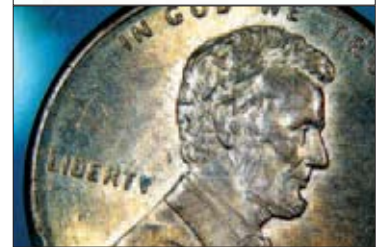
Stage 3 incident light: the lower two LEDs light finely structured objects from a low level, increasing contrast.
