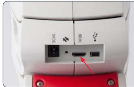
2. Connect the HDMI cable to the HDMI television or monitor.
