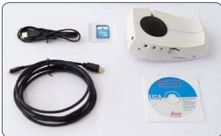
*The contents include the camera module, CD with imaging software, SD Card, HDMI and USB cable.*
