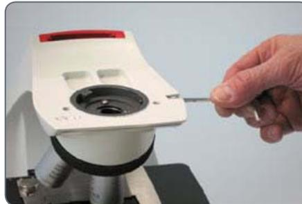
3. Insert the dovetail (see the underside of the Leica ICC50 HD) into the stand support.
