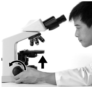
Raise the stage until this distance is slightly smaller than the working distance.
