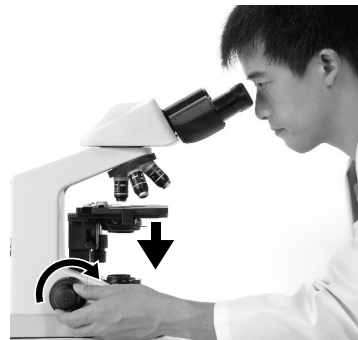
Lower the stage with the fine focus knob to find the focal point.
