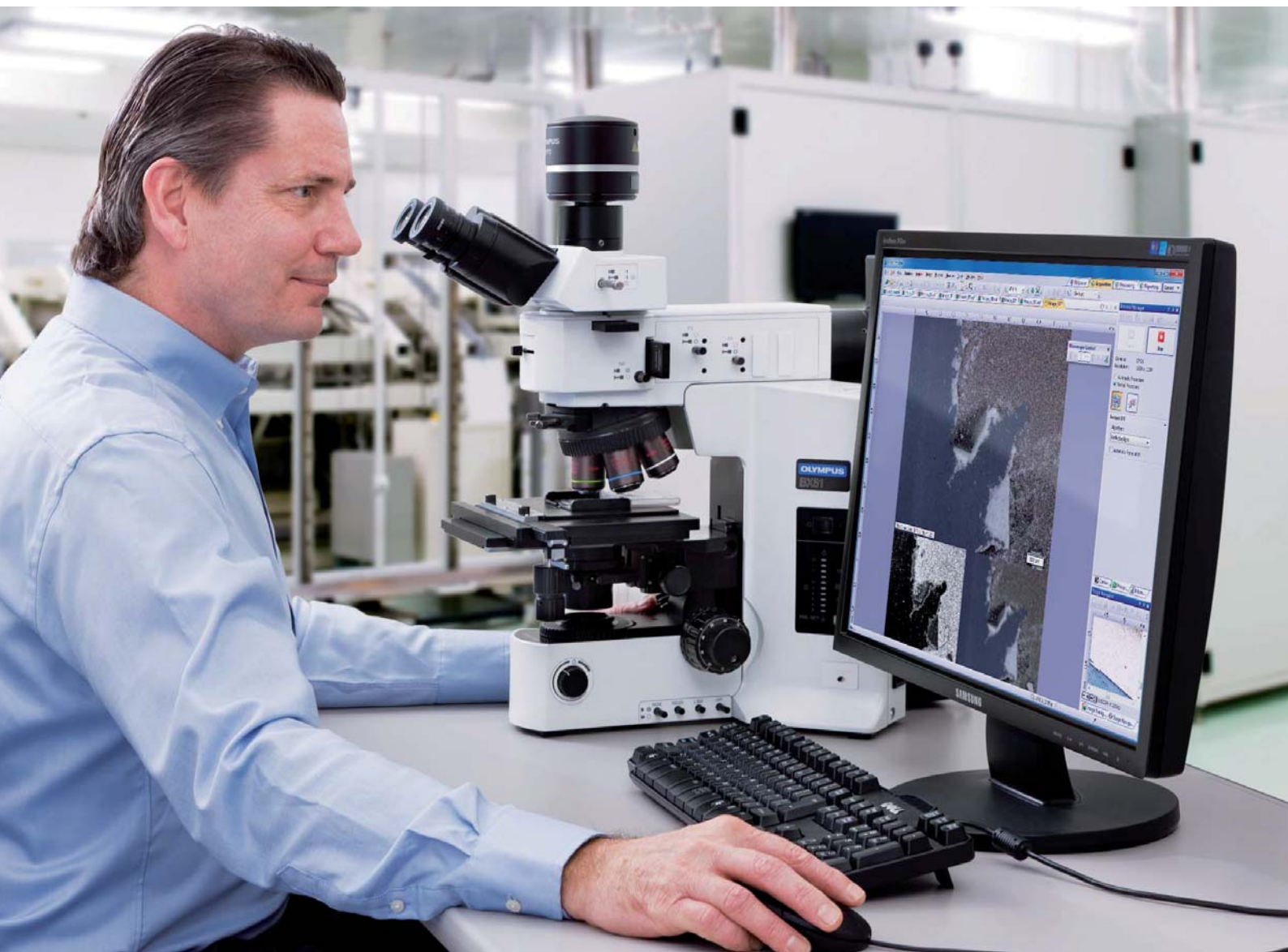
Easy-to-use design (e.g. tilting tube and fine focusing knob attaches to either side)
