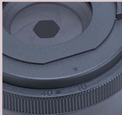
Field diaphragm with position guide markings
