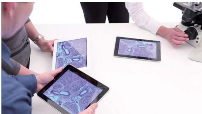
Multiple iPad can be connected to the same camera so that the user can share live images.
