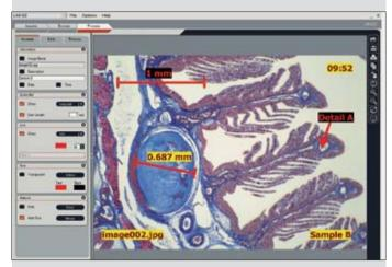
Process: After image capture you can easily add annotations and basic measurements to the images. A gallery of images stores all the calibration and camera data for fast reference.
