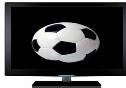
4:3 aspect ratio image on a screen set to an aspect ratio of 16:9
