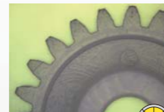
Resin parts (optical magnification 0.35x) Type A zooming head / 8 segment LED ring light
