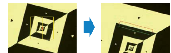
The search probe can detect misaligned parts, and rotate the program to suit. Allowing the machine to successfully measure the part.
