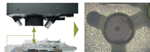
Working distance 73.5mm Assembled components Under coaxial top light at 0.35x optical magnification
