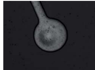
High density PCB Under coaxial top light at optical magnification 4x
