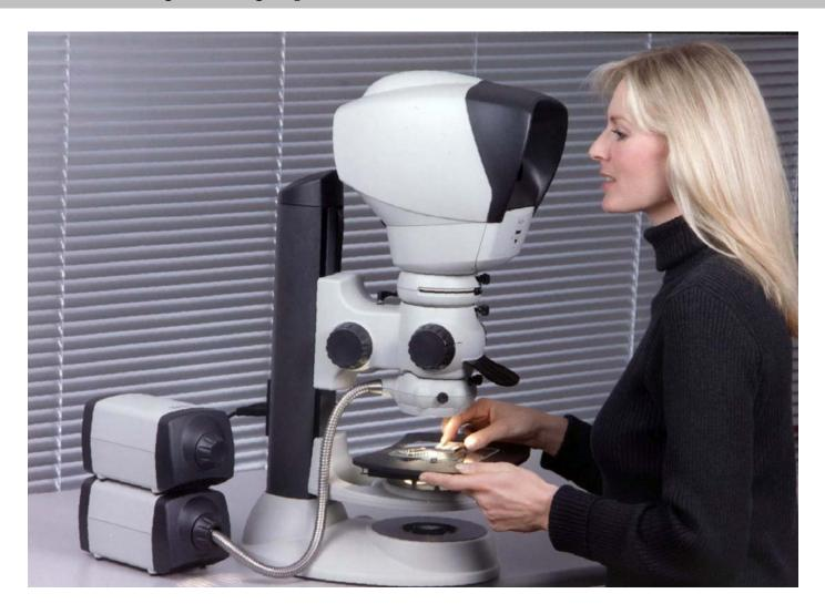
The eyepieceless viewer enables unmatched freedom of head and body position, eliminating operator fatigue, due to an exit pupil 64x larger than traditional eyepiece microscopes. This produces a high-resolution image over a large viewing area.
