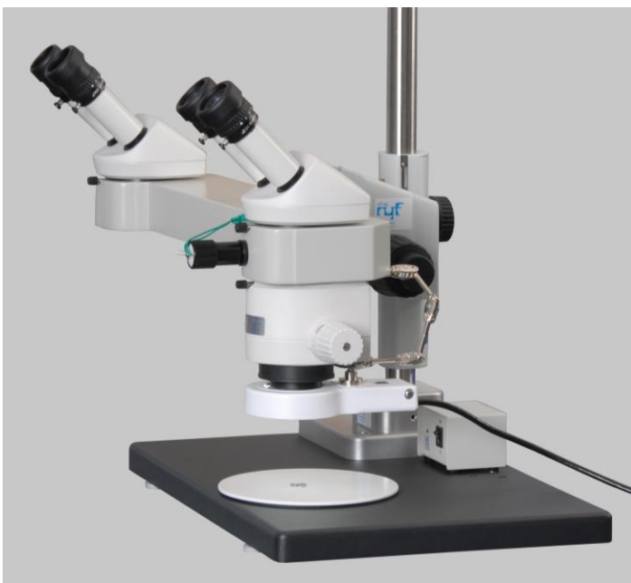
Version DSK-FOF-MZ with zoom 6.3x – 40x and Ryf NKL 18 illuminator
