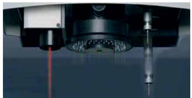
Measuring head of the PMS Series with a CCD matrix camera, a TP 200 touch probe which retracts after use and a conoscopic measuring laser.
