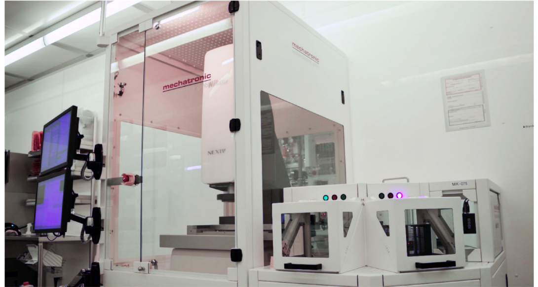
Nikon Metrology NEXIV VMZ-R3020, automated with an mWL150 Single-Arm Wafer Handling Tool. This is the first system to be installed in a cleanroom at the Nuremberg plant of Semikron Elektronik GmbH.
