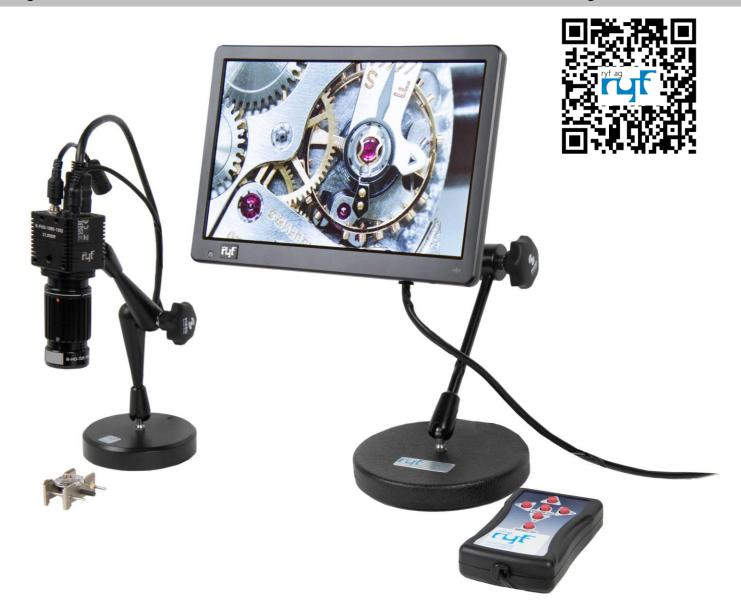
Full-HD mini video camera system as a «replacement» for a stereo microscope
