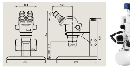
Trinocular version: with C-PS tripod, Ryf NKL12 LED illumination with built-in diffuser and camera.
